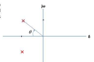
• For Underdamped system  $0^{\circ} < \theta < 90^{\circ}$  therefore,  $0 < \zeta < 1$
