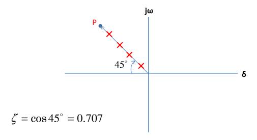
• Therefore, s-plane is divided into sections of constant damping ratio lines.
