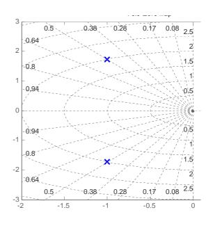
Determine the location of closed loop poles so that the damping ratio remains same but the natural undamped frequency is doubled.
