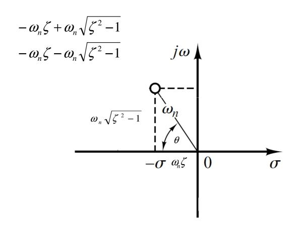
$$\frac{C(s)}{R(s)} = \frac{\omega_n^2}{s^2 + 2\zeta\omega_n s + \omega_n^2} \xrightarrow{\text{Step Response}} C(s) = \frac{\omega_n^2}{s(s^2 + 2\zeta\omega_n s + \omega_n^2)}$$
