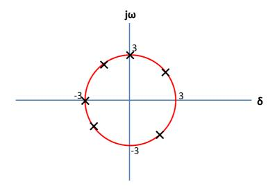
• Therefore the s-plane is divided into Constant Natural Undamped Frequency  $(\omega_n)$  Circles.
